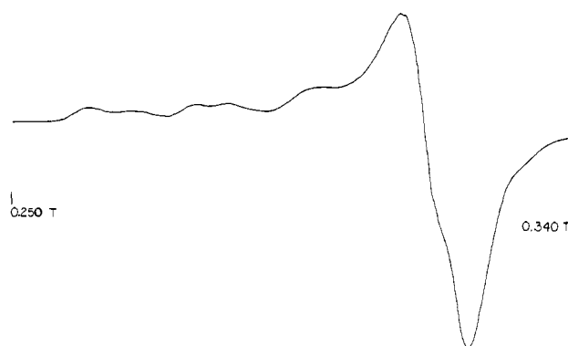
Figure 3. Experimental EPR spectrum of 4% copper-doped nickel-bacitracin A powder. Instrument parameters: \nu = 9.11564 GHz, 90-mT scan range centered at 295.0 mT, time constant = 0.03 s, 4-min scan, 0.10 mT peak-to-peak modulation at 100 kHz, microwave power = 3.0 mW, receiver gain = 630, temperature = 77 K.
